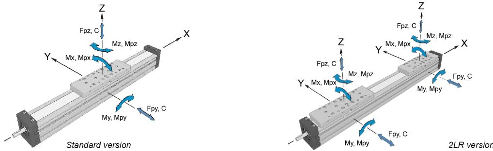
The stated values are for strokes up to 500 mm. No load torque value increases with stroke elongation.
