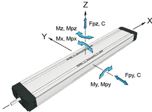
For length/stroke over the stated value, please contact Rollco. Values for max. stroke are not valid for double carriage (equation of defining the linear unit length for particular size of the linear unit needs to be used).
