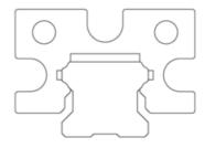
\* MF contact surfaces are tolerance match to the guiderail to ensure perfect sealing
