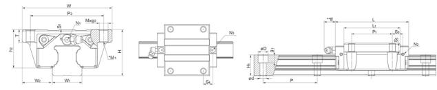
\*M1: Bolt size for bottom mounting type of block \*\*E: Size 15 delivered with straight standard nipple. Size 20 – 55 delivered with angled standard nipple.
