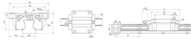
\*M1: Bolt size for bottom mounting type of block \*\*E: Size 15 delivered with straight standard nipple. Size 20 – 55 delivered with angled standard nipple.
